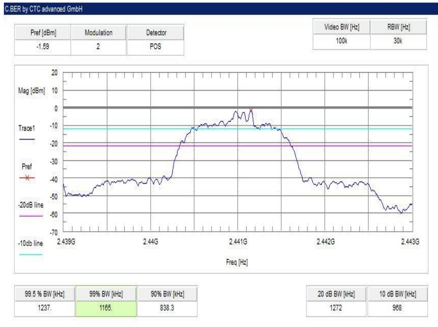
Plot 8: middle channel – 2441 MHz, 8 DPSK modulation
