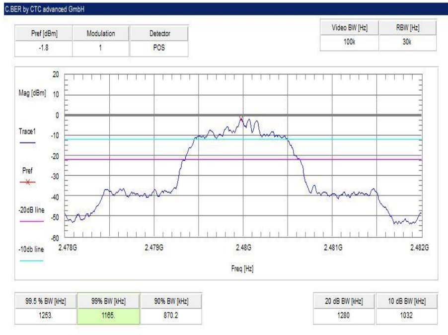
Plot 6: highest channel – 2480 MHz, Pi / DQPSK modulation
