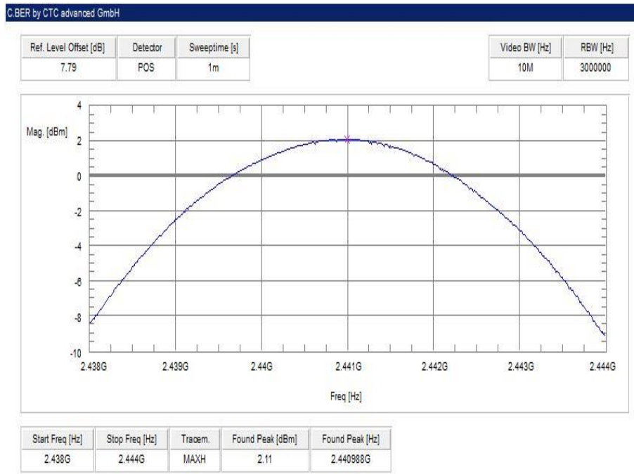
Plot 8: middle channel – 2441 MHz, 8 DPSK modulation
