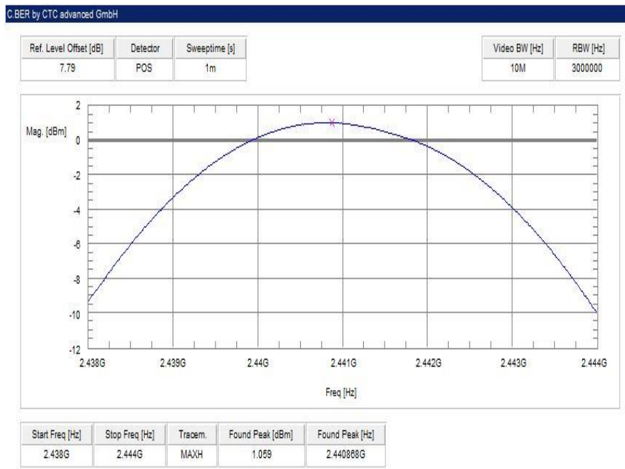
Plot 2: middle channel – 2441 MHz, GFSK modulation
