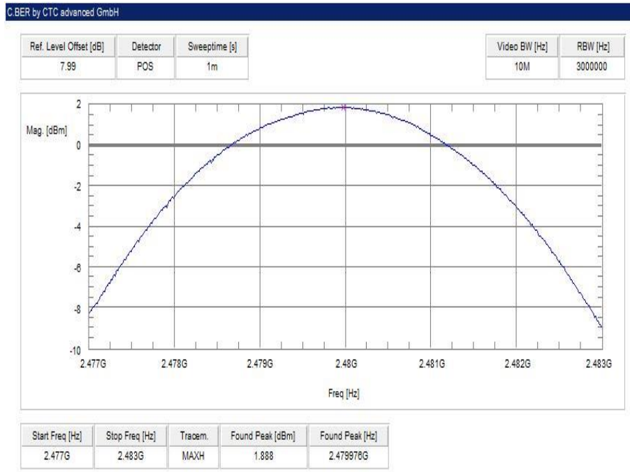
Plot 9: highest channel – 2480 MHz, 8 DPSK modulation
