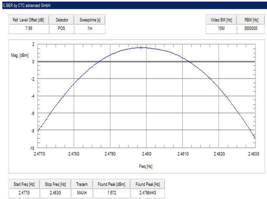
Plot 6: highest channel – 2480 MHz, Pi / DQPSK modulation
