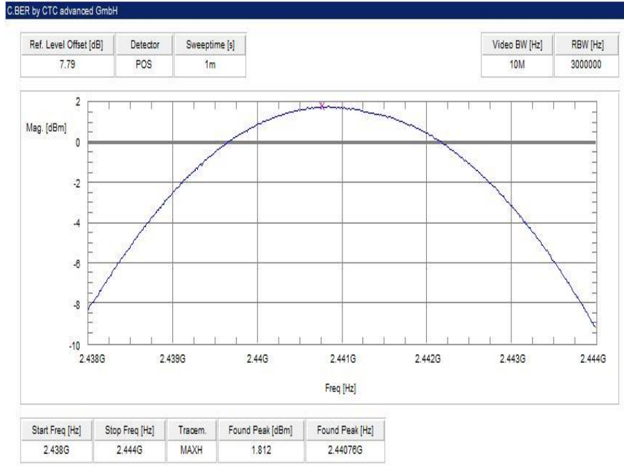
Plot 5: middle channel – 2441 MHz, Pi / DQPSK modulation
