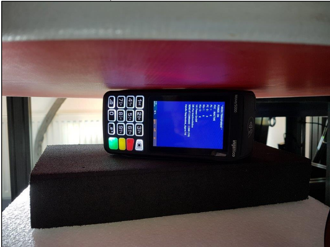
Photo 12: Test position limb worn right side with 0 mm distance
