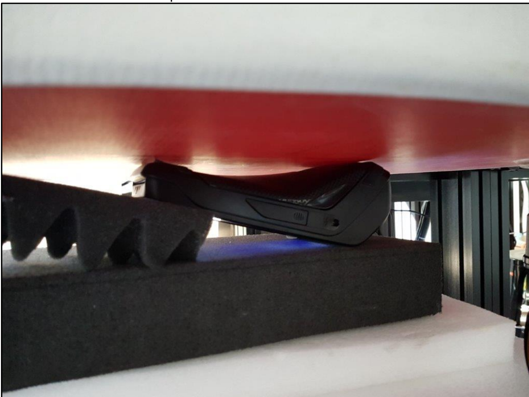
Photo 10: Test position limb worn back side with 0 mm distance
