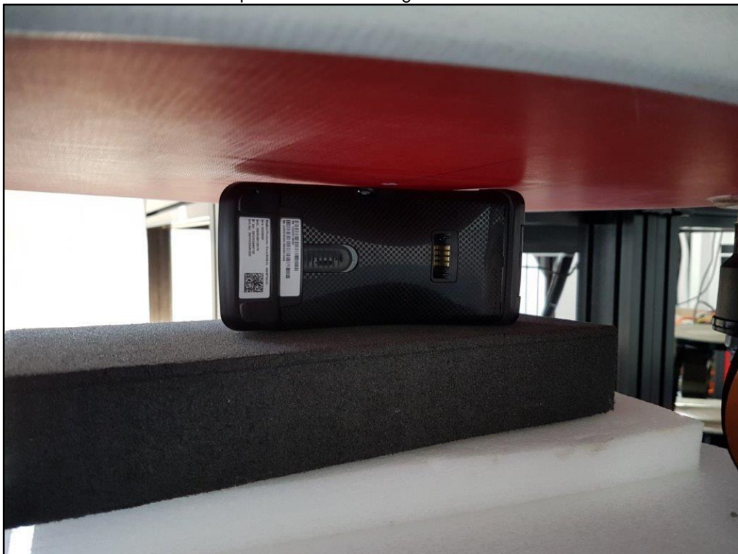
Photo 12: Test position limb worn right side with 0 mm distance
