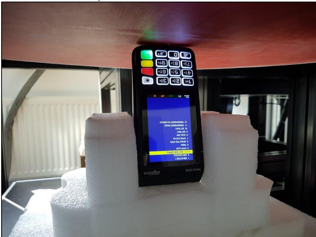
Photo 14: Test position limb worn bottom side with 0 mm distance
