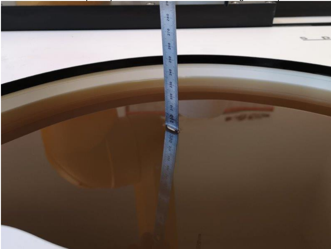
Photo 1: Liquid depth HBBL600-10000MHz Simulating Head Liquid
