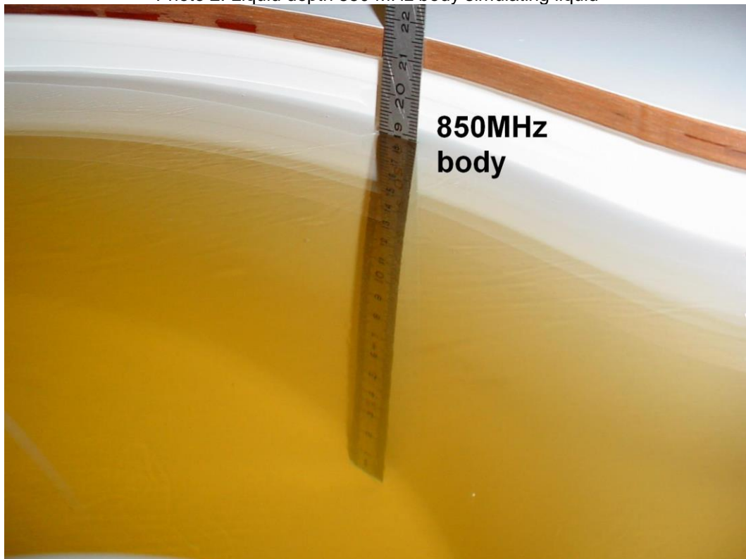
Photo 2: Liquid depth 850 MHz body simulating liquid
