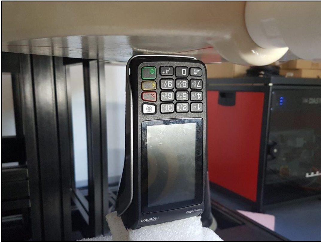
Photo 13: Test position bottom side without any distance
