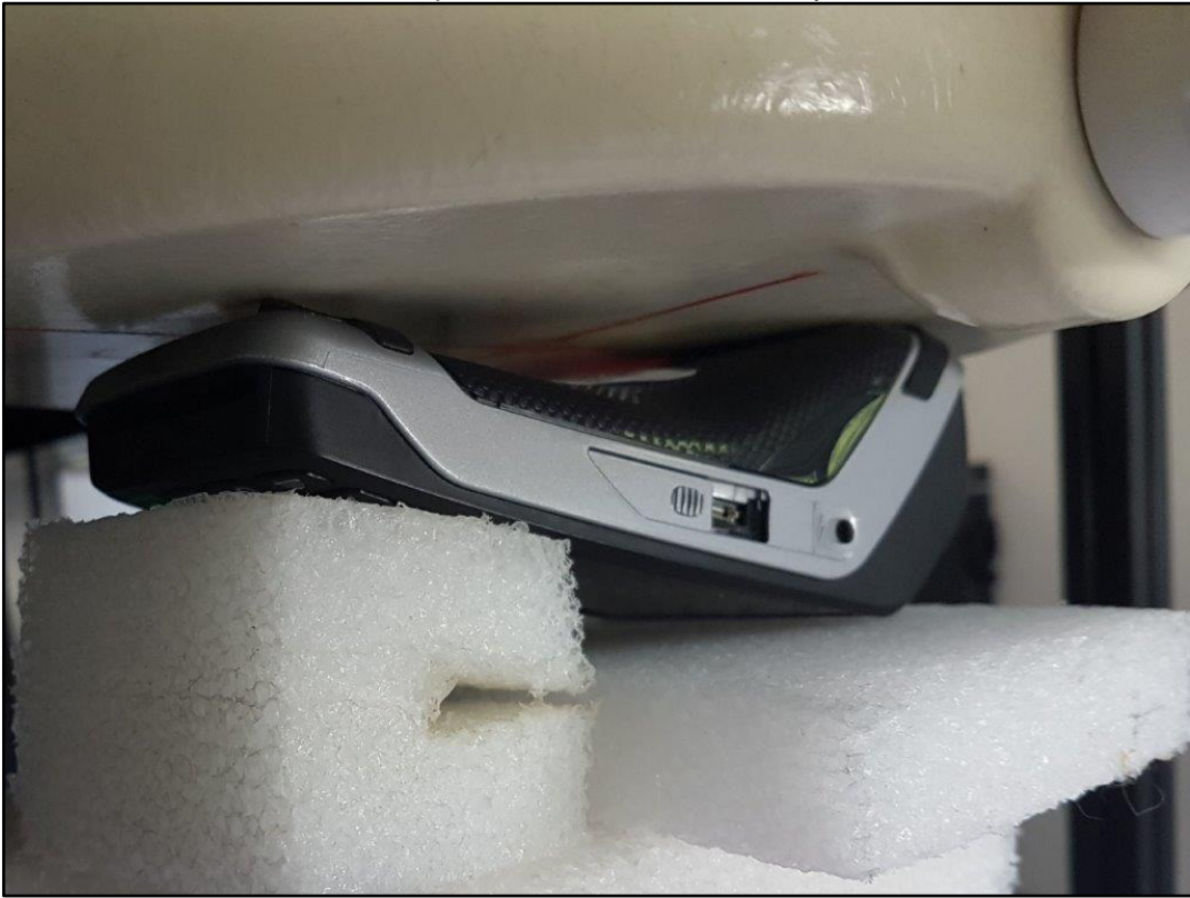
Photo 10: Test position left side without any distance
