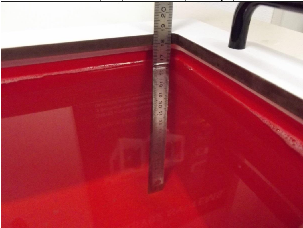
Photo 2: Liquid depth 1900 MHz body simulating liquid
