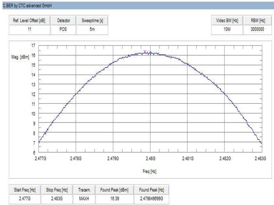
Plot 6: highest channel – 2480 MHz, Pi / DQPSK modulation
