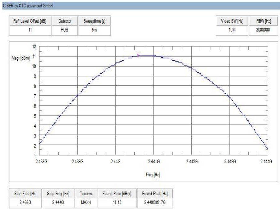
Plot 2: middle channel – 2441 MHz, GFSK modulation
