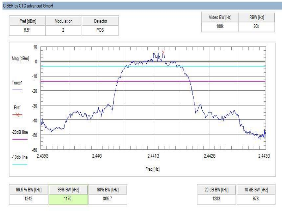
Plot 8: middle channel – 2441 MHz, 8 DPSK modulation
