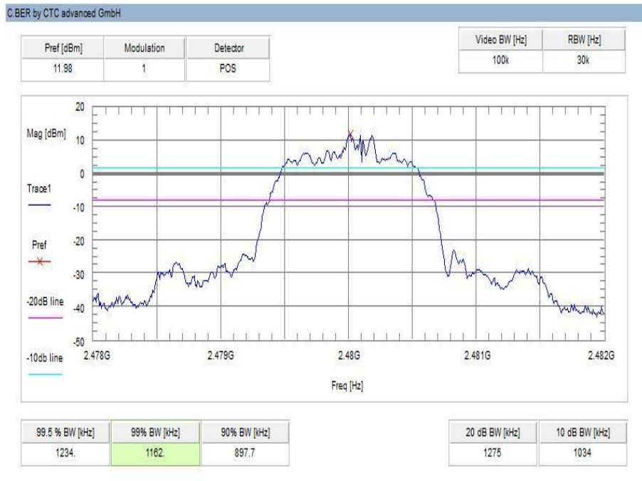
Plot 6: highest channel – 2480 MHz, Pi / DQPSK modulation
