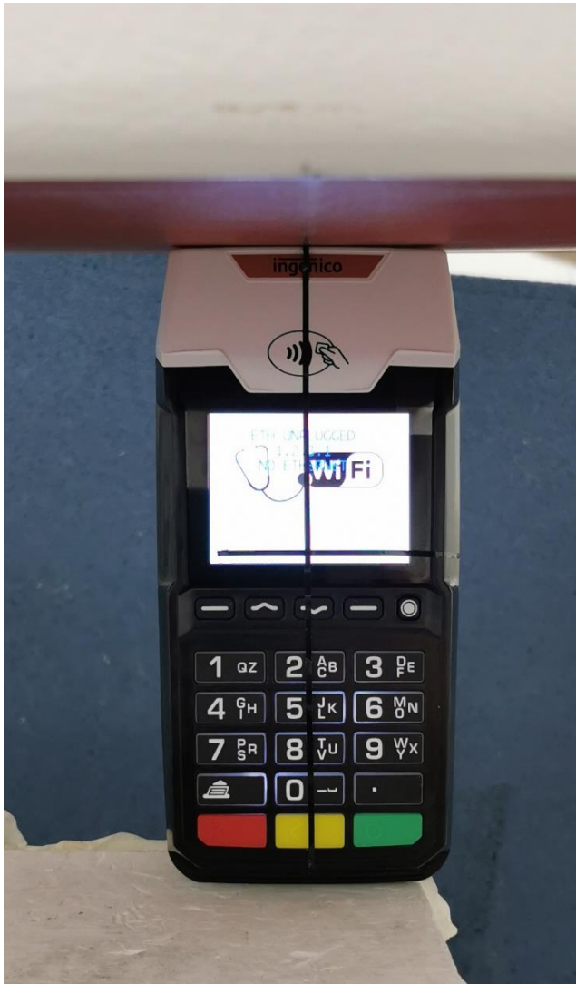
Figure 6 Top test position, 0mm separation distance
