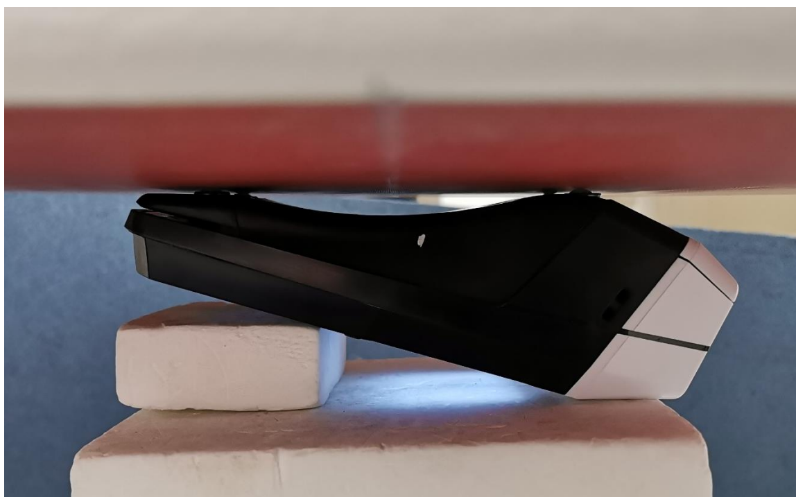
Figure 3 Back test position, 0mm separation distance
