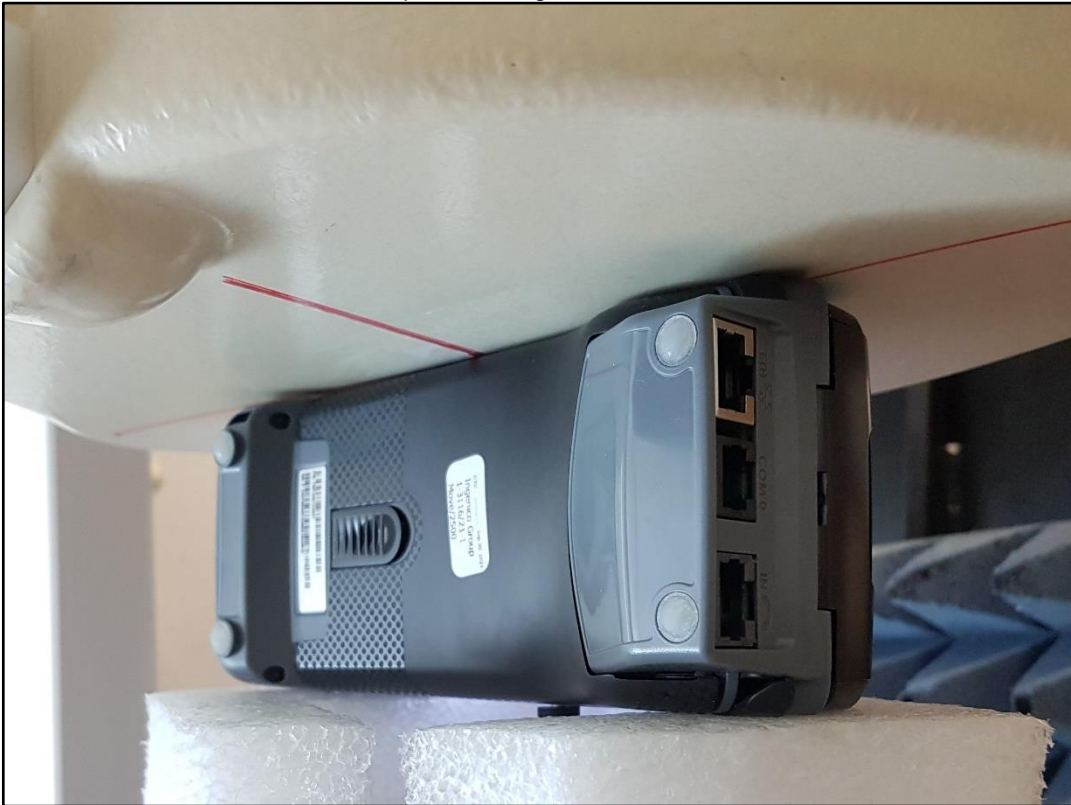
Photo 12: Test position - left side with 0mm distance
