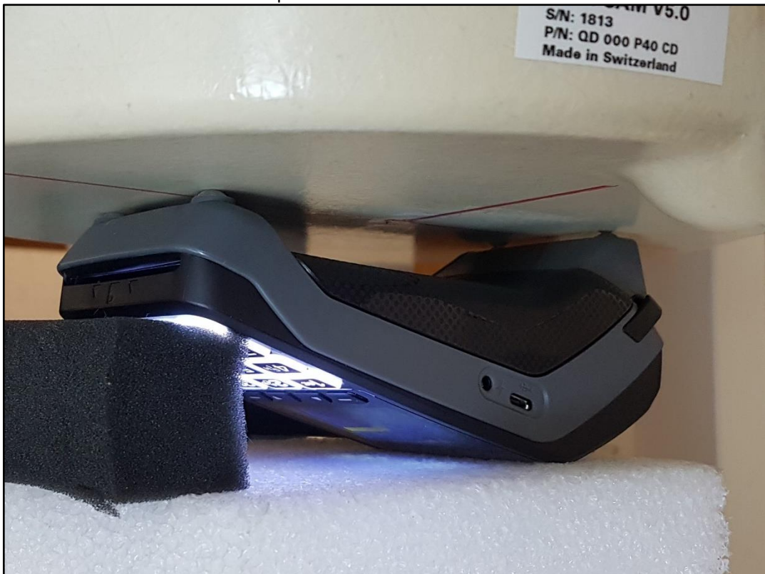
Photo 10: Test position - Bottom side with 0mm distance
