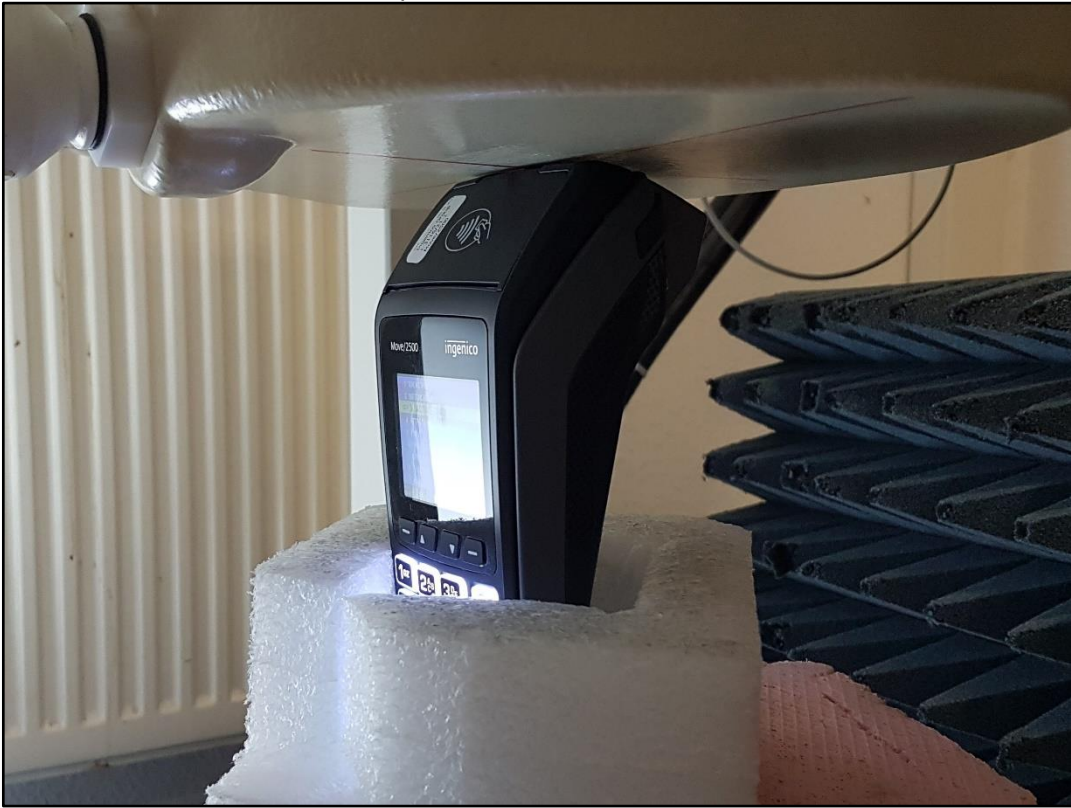
Photo 14: Test position - Front side with 0mm distance
