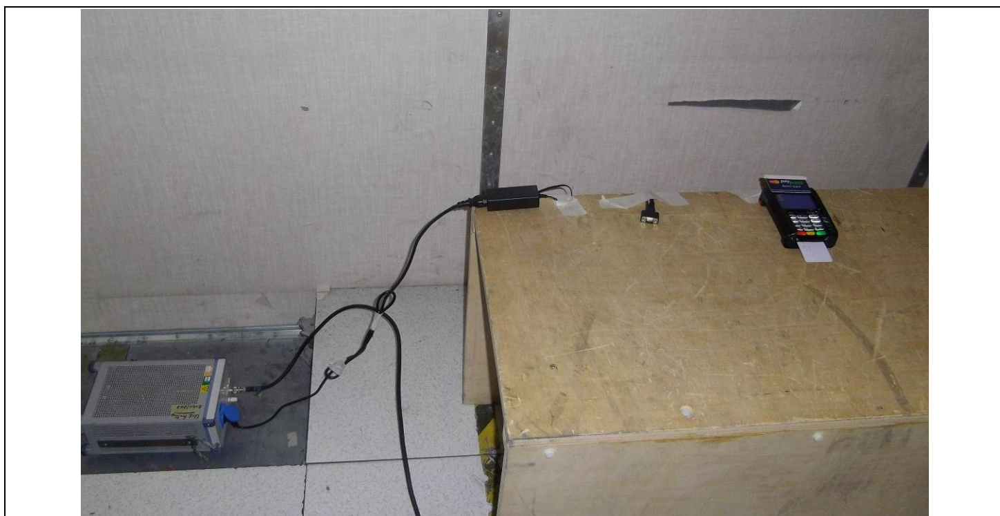
Photograph for AC Power Line Conducted Emissions (Global view)
