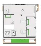
Insert the SAM Card into the slot marked (1), (2) or (3) by sliding it. Take care to ensure that the SAM Card is inserted in the correct manner. The cut corner must be positioned as indicated on the figure below.
