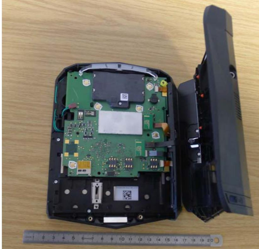
Photo 1 (EUT rear view – rear cover removed):
