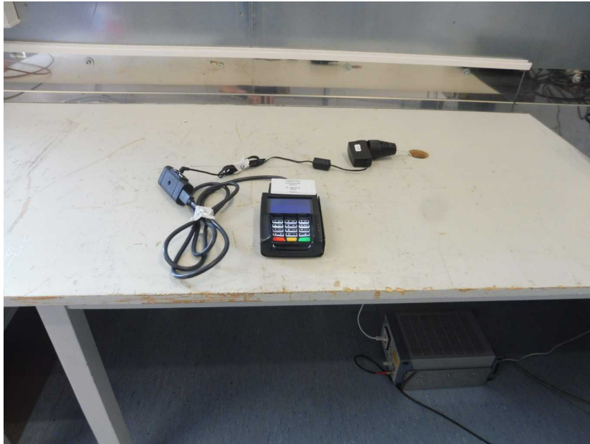
Photo 7: AC conducted test setup
