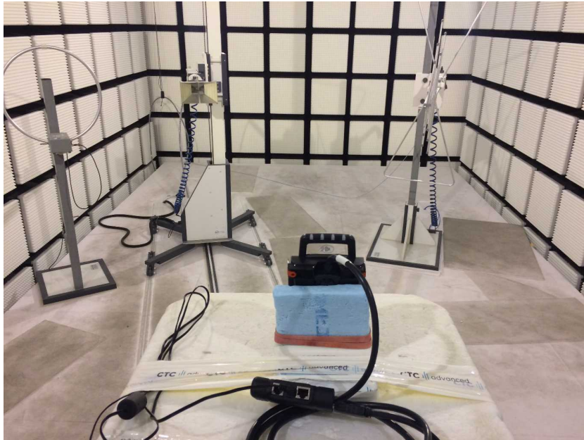
Photo 3: RSE test setup >1GHz
