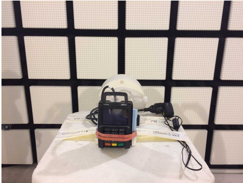
Photo 1: RSE test setup >1GHz
