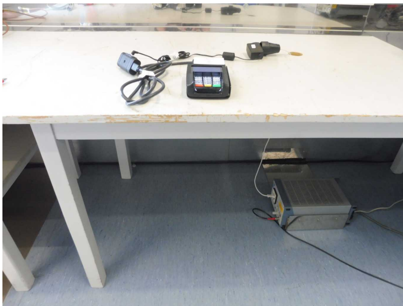
Photo 8: AC conducted test setup
