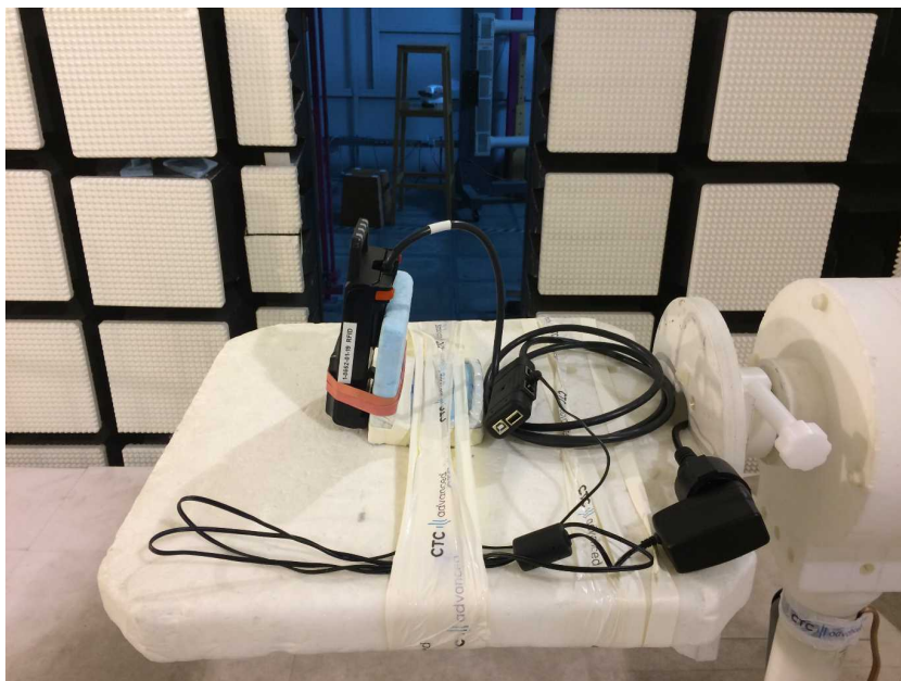
Photo 2: RSE test setup >1GHz
