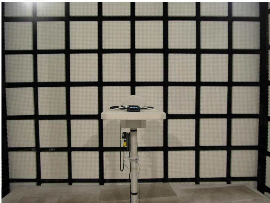
Photo 4: EUT at the anechoic chamber
