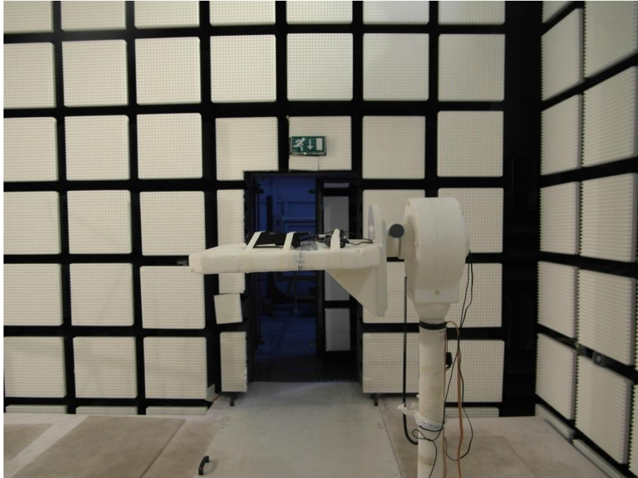
Photo 3: EUT at the anechoic chamber
