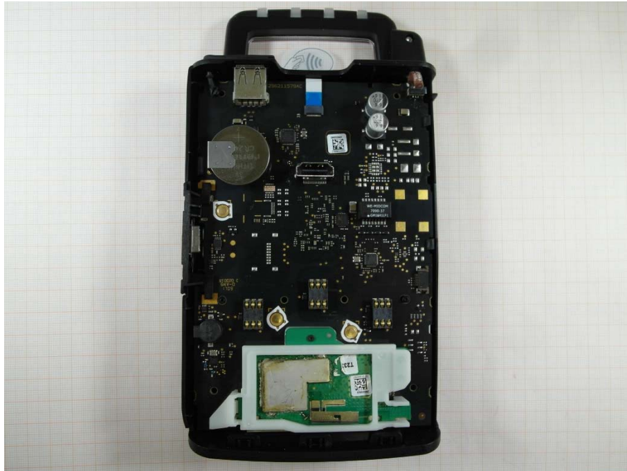
Photo 3: PCB with RF module in the bottom
