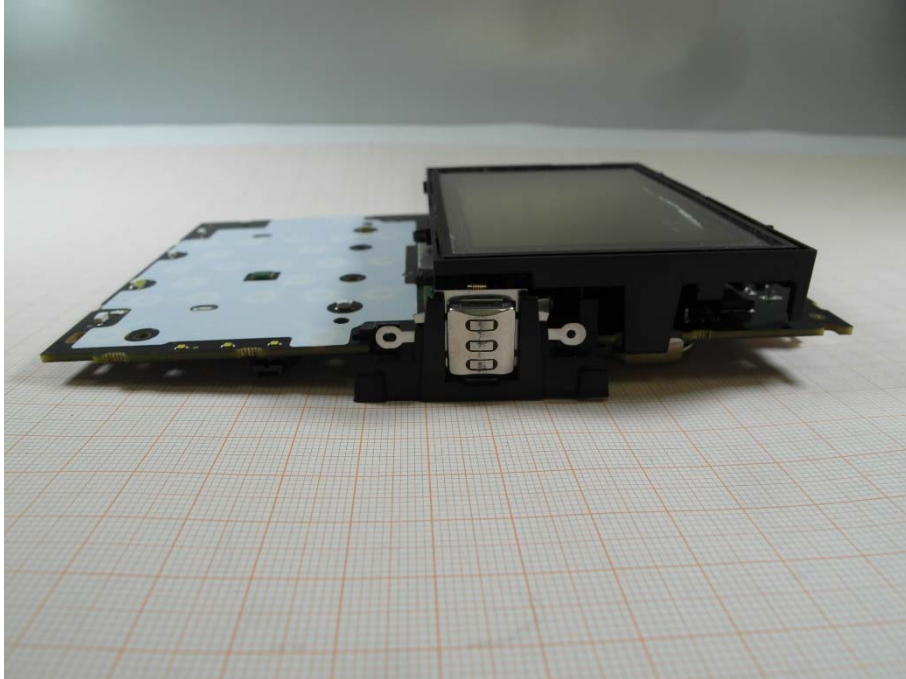
Photo 7: right side view on PCB with display and card reader
