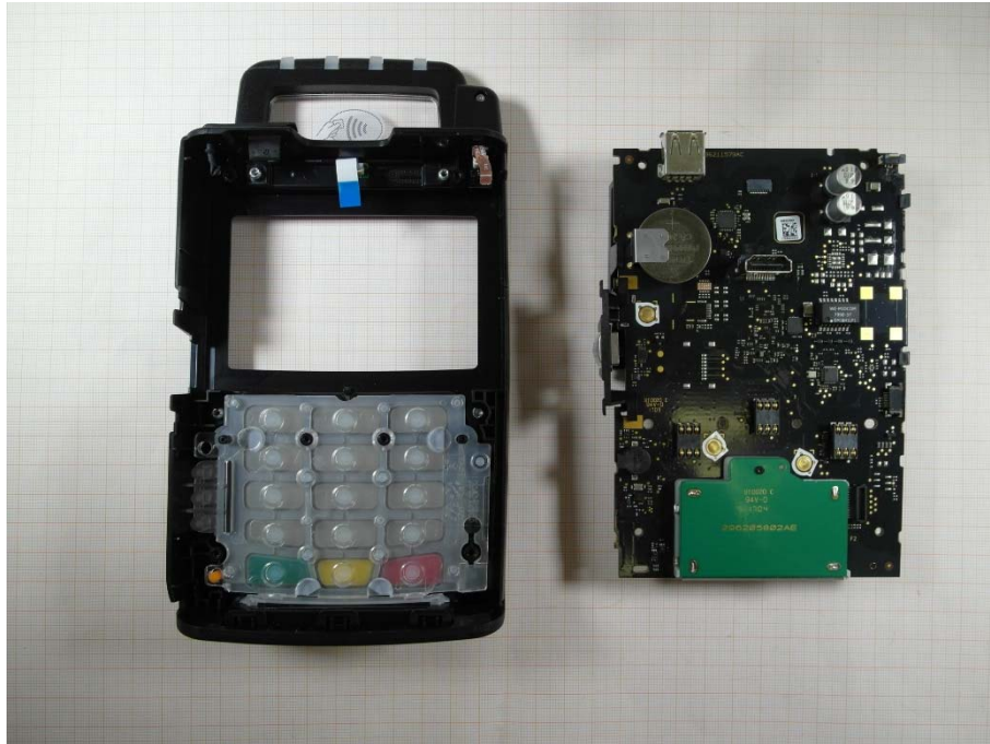
Photo 5: PCB removed from case
