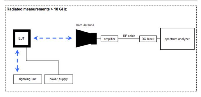
Measurement distance: horn antenna 50 cm
