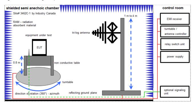
Measurement distance: tri-log antenna 10 meter
