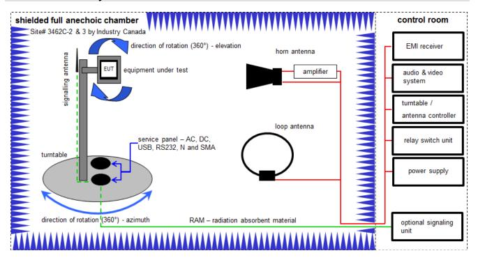
Measurement distance: horn antenna 3 meter; loop antenna 3 meter
