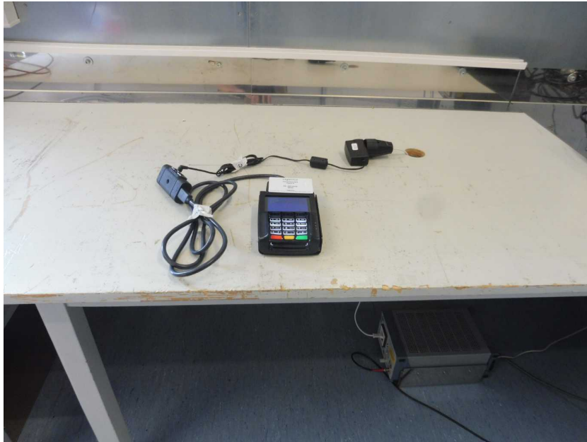
Photo 7: AC conducted test setup
