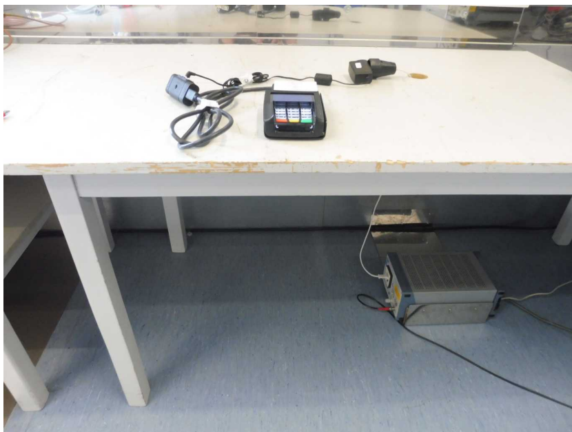
Photo 8: AC conducted test setup
