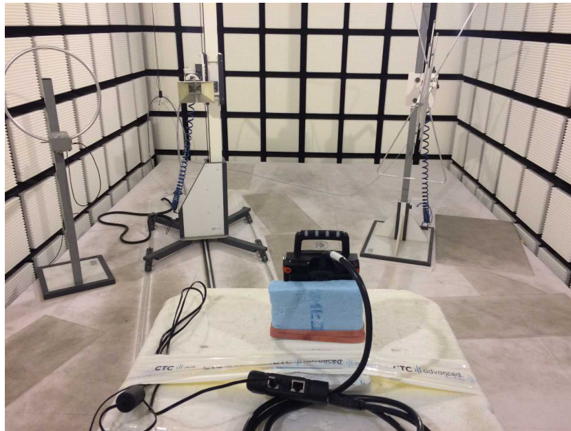
Photo 3: RSE test setup >1GHz
