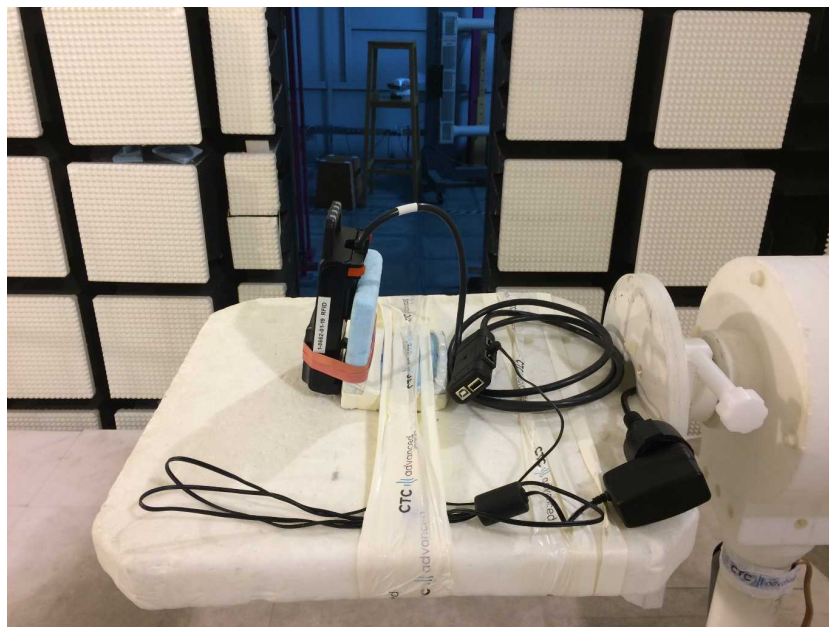
Photo 2: RSE test setup >1GHz
