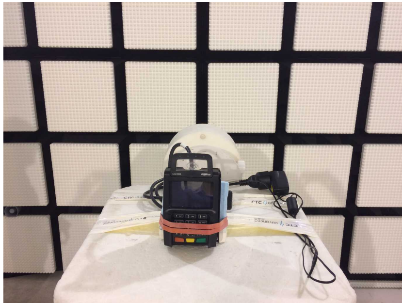
Photo 1: RSE test setup >1GHz
