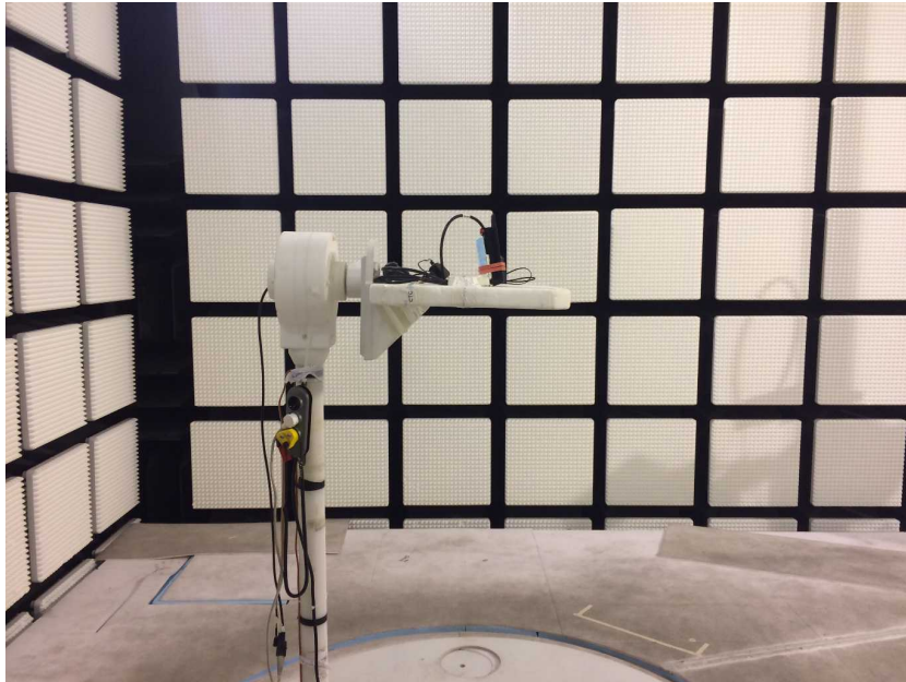
Photo 5: RSE test setup >1GHz
