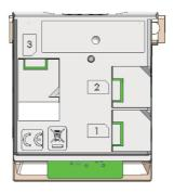
Insert the SAM Card into the slot marked (1), (2) or (3) by sliding it. Take care to ensure that the SAM Card is inserted in the correct manner. The cut corner must be positioned as indicated on the figure below.
