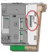
• Slide back the module inside the terminal and screw it tight
