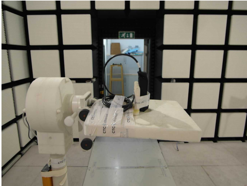
Photo 3: EUT at the anechoic chamber
