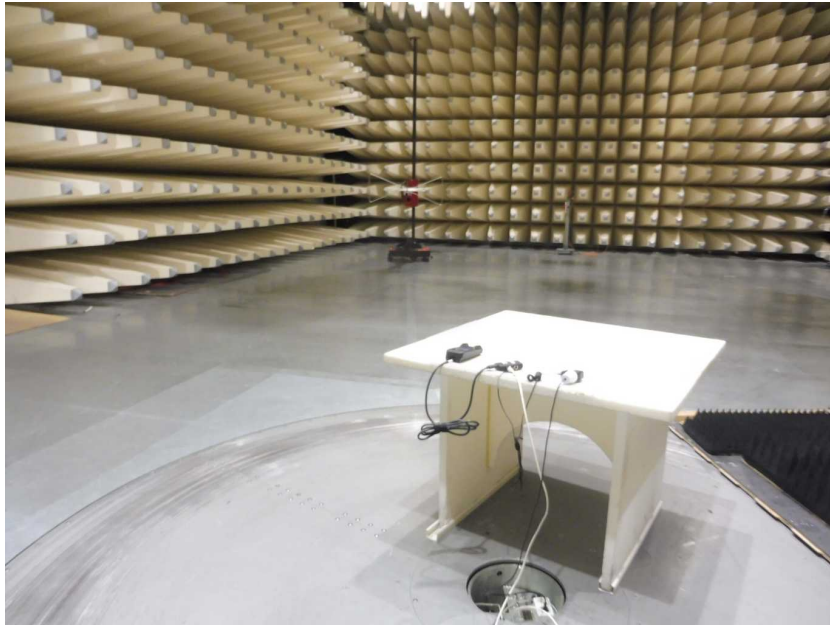
Photo 7: EUT at the semi-anechoic chamber
