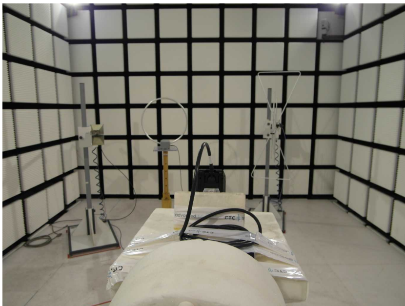
Photo 4: EUT at the anechoic chamber
