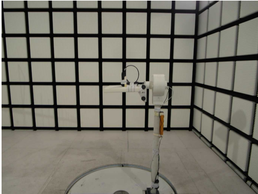
Photo 5: EUT at the anechoic chamber
