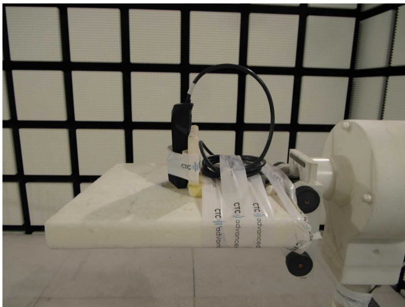
Photo 2: EUT at the anechoic chamber
