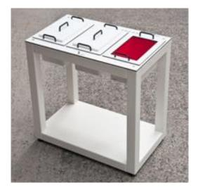
Triple Modular Phantom consists of three identical modules which can be installed and removed separately without emptying the liquid. It includes three reference points for phantom installation. Covers prevent evaporation of the liquid. Phantom material is resistant to DGBE based tissue simulating liquids.
