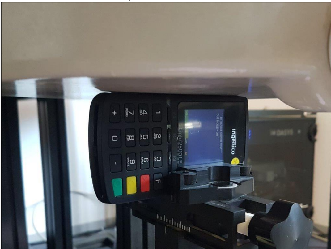
Photo 12: Test position left side with 0 mm distance
