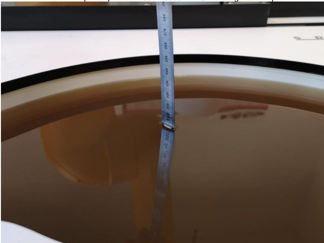
Photo 2: Liquid depth HBBL600-10000MHz Simulating Head Liquid
