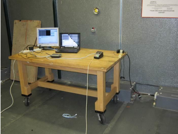
Figure 8 Test Setup for Conducted Emissions
