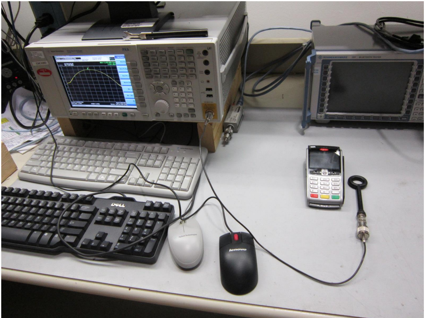
Figure 10 Test Setup for Occupied Bandwidth
