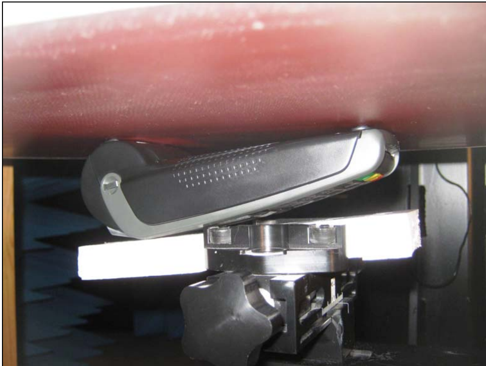
Fig. 4: Rear side at 0cm from the phantom
