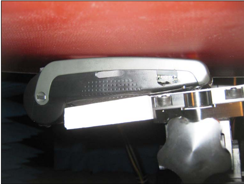
Fig. 3: Front side at 0cm from the phantom
