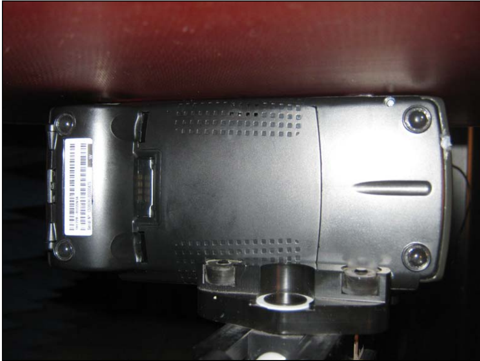
Fig. 5: Left side at 0cm from the phantom
