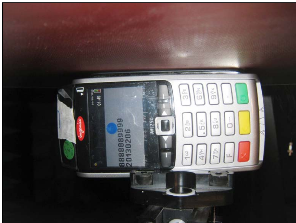
Fig. 16: Right side at 0cm from the phantom
