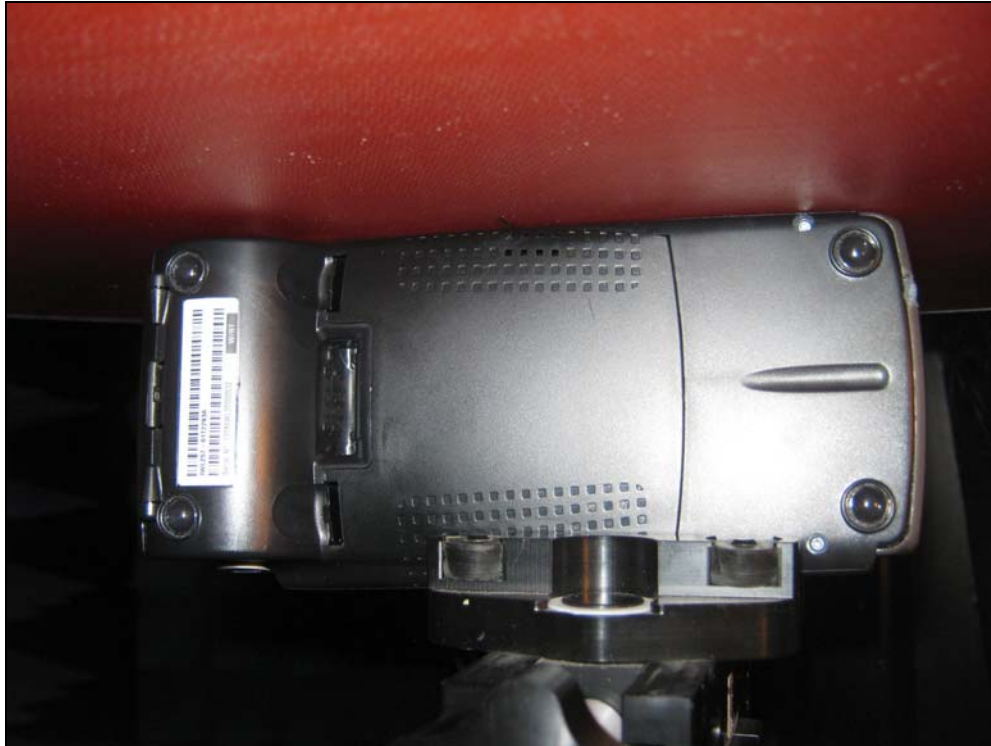
Fig. 15: Left side at 0cm from the phantom
