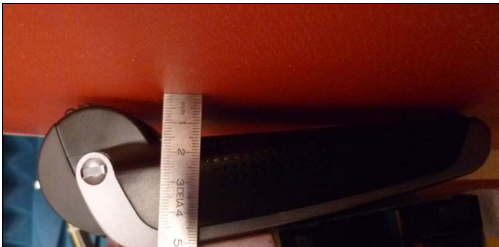
Fig. 14: Distance from the phantom when rear side is positioned at 0cm
