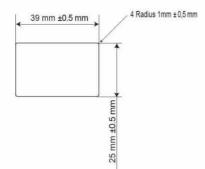
Color: White RAL9010 Adhésive one side: permanent UL969 certified Material: Vynil or Polyester, thickness 50 to 100µm UL969 certified
