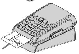
• <u>2<sup>nd</sup> card reader (Optional)</u>: is located under terminal trapdoor (on back of the terminal). Insert the card up side down, magnetic stripe visible.
