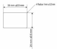
Color: White RAL9010 Adhésive one side: permanent UL969 certified Material: Vynil or Polyester, thickness 50 to 100µm UL969 certified
