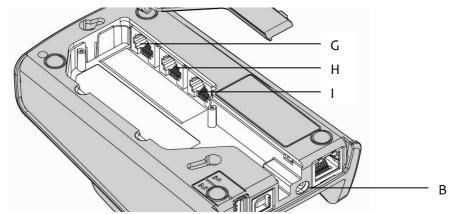
G= Serial link COMØ – RS232 (optional)H= Serial link COM1 – RS232 (optional)I = Modem socket (optional)
