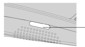
USB (microAB) Connector used for PC, travel charger adapter, USB Key, etc...)
