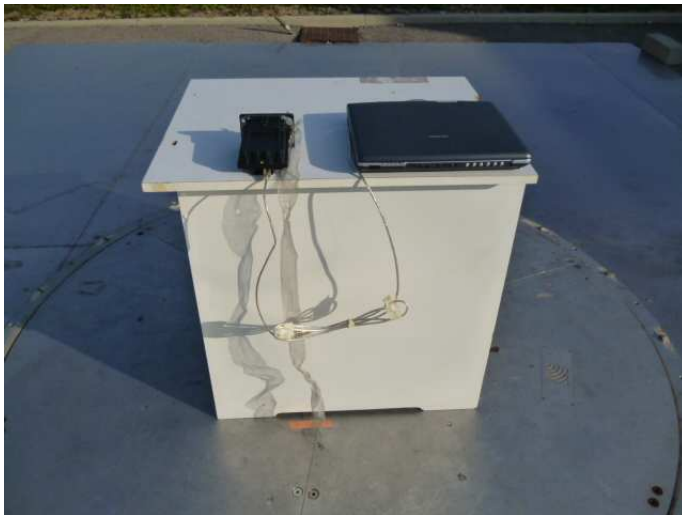
Radiated emission test setup
