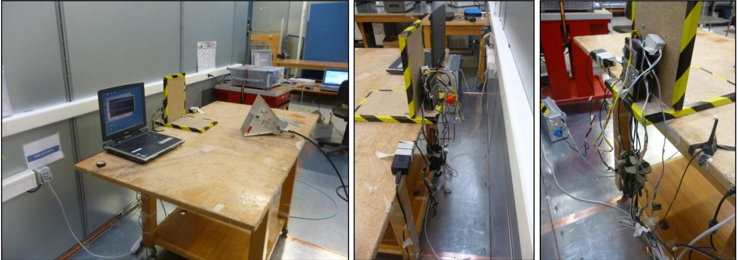
Conducted emission test setup
