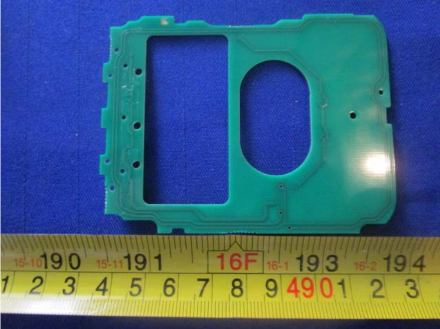
EUT- Antenna Board Bottom View
