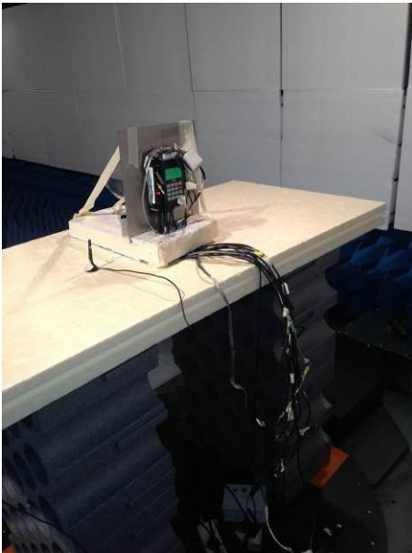
Radiated emission test setup
