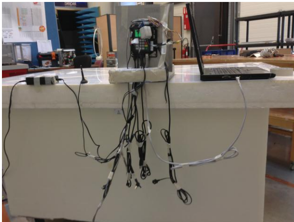
Conducted emission test setup
