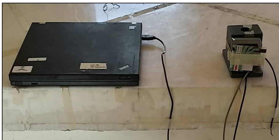
Test setup on OATS – Worst case
