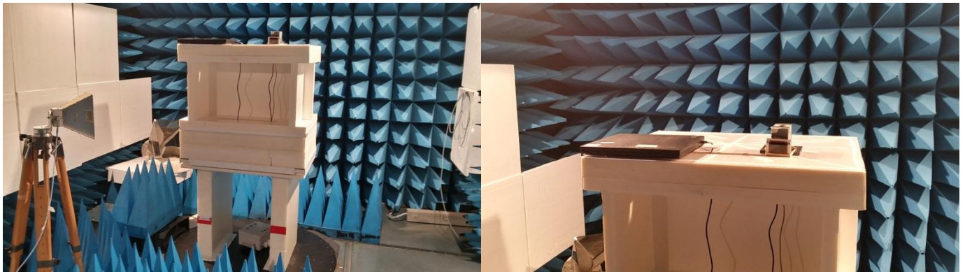
Test setup in anechoic chamber (Pos Z) – setup >1GHz
