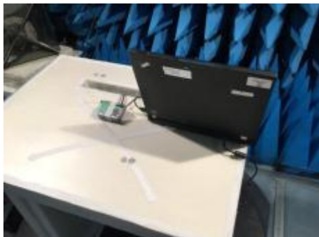
Test setup in anechoic chamber (Configuration2 and axis XZ)
