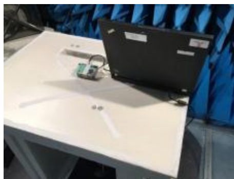
Test setup in anechoic chamber (Configuration1 and axis Z)
