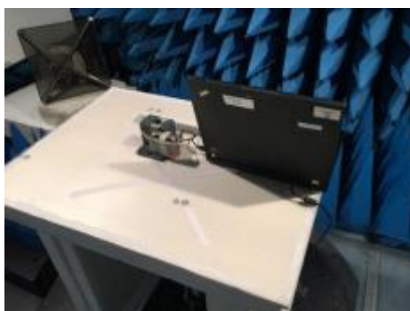
Test setup in anechoic chamber (Configuration2 and axis Z)
