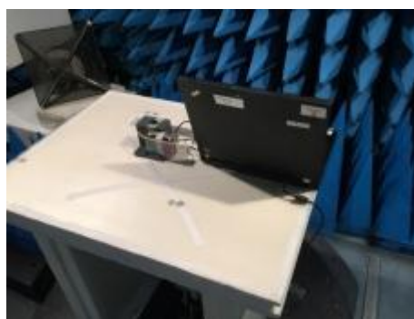
Test setup in anechoic chamber (Configuration1 and axis Z)
