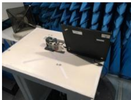
Test setup in anechoic chamber (Configuration2 and axis Z)
