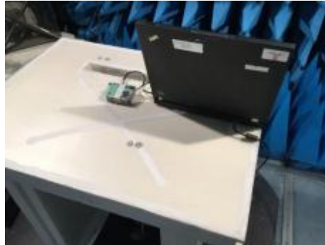
Test setup in anechoic chamber (Configuration1 and axis Z)
