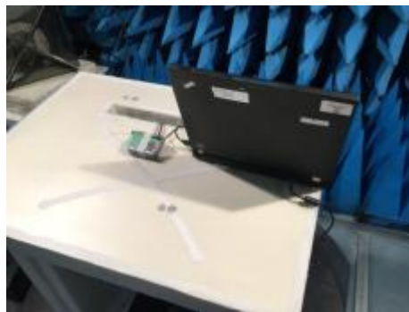
Test setup in anechoic chamber (Configuration2 and axis XZ)
