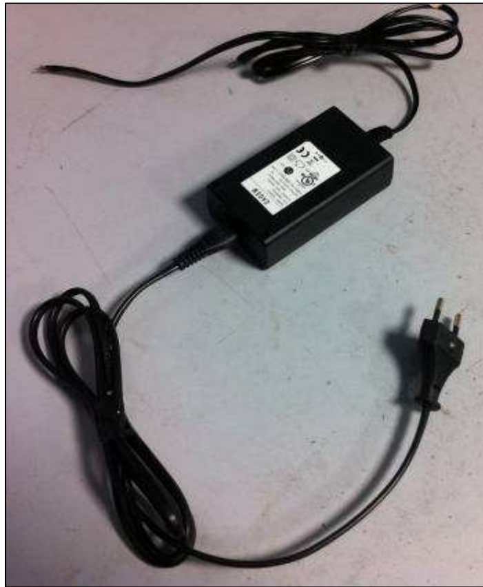
Power supply SAGEM AD5632 (Configuration n2), "Used to emulate a 8Vdc power source"
