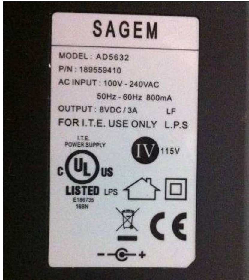
Power supply SAGEM AD5632 (Configuration n2), "Used to emulate a 8Vdc power source"
