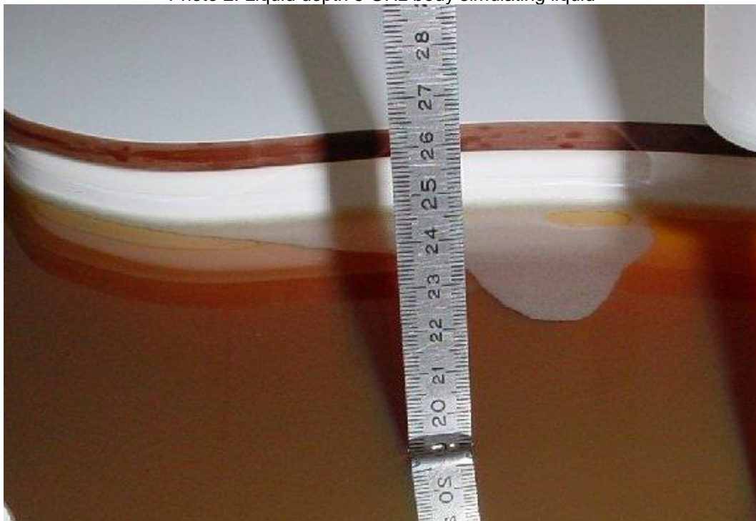
Photo 2: Liquid depth 5 GHz body simulating liquid
