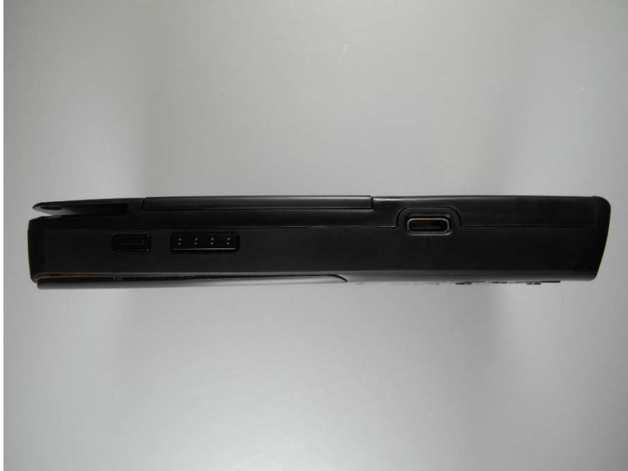
Photo 5: right side with USB interface
