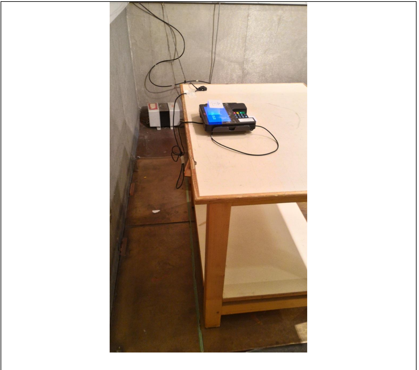
Test set up of conducted emission on power supply
