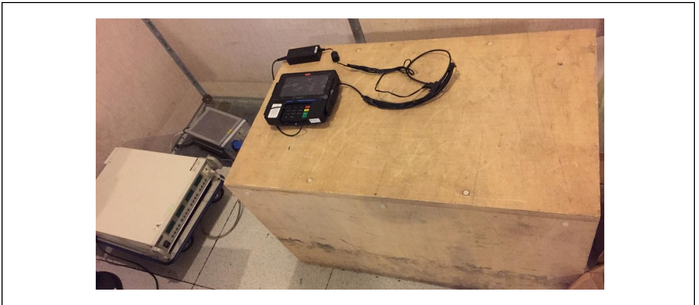
Test set up of conducted emission on power supply
