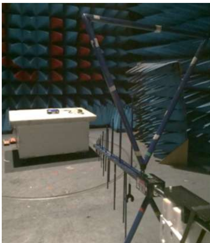
Radiated emissions measurements
