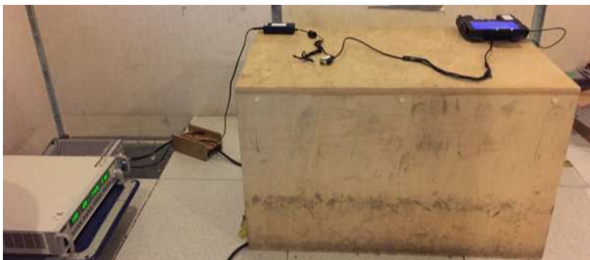
Conducted emission measurements
