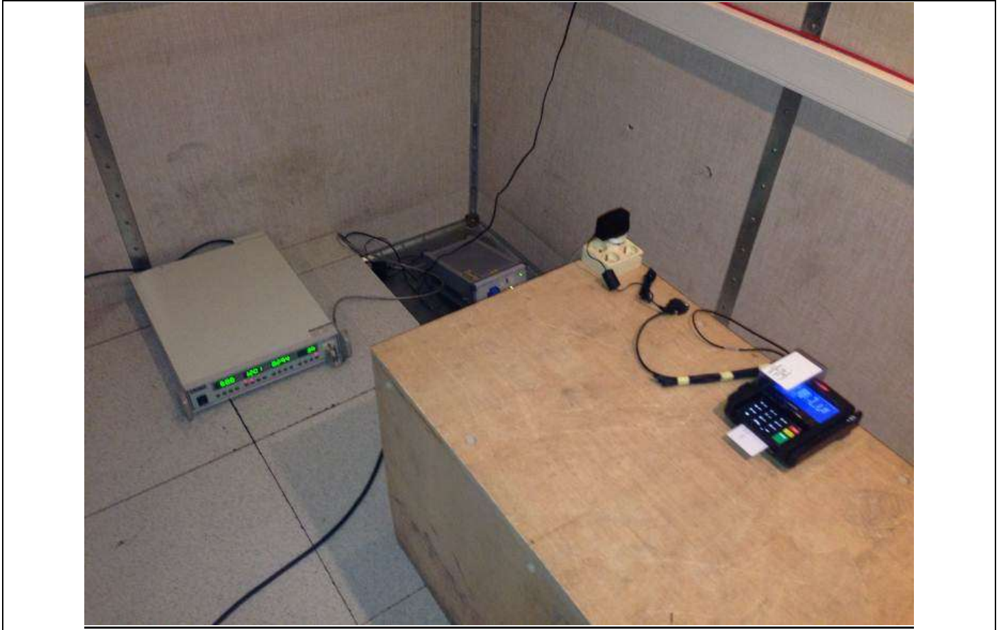
Photograph for AC Power Line Conducted Emissions (Global view)
