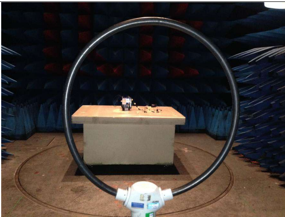
Photograph for Field strength within the band 13.110-14.010MHz
