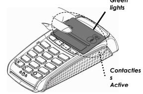
When a contactless card is presented to the contactless active zone during a transaction the second, third and fourth status lights will be lit in turn. The card read is successful when all four status lights are lit and the confirmation tone is heard.
