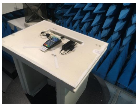
General Test setup in anechoic chamber
