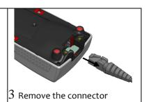
1 Remove the cable flap by clamping the<br/>slot as indicated by the arrows2 Press thTo connect the cable, proceed in reverse order.
