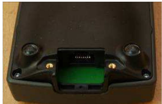
RJ45 Connector without plastic cover
