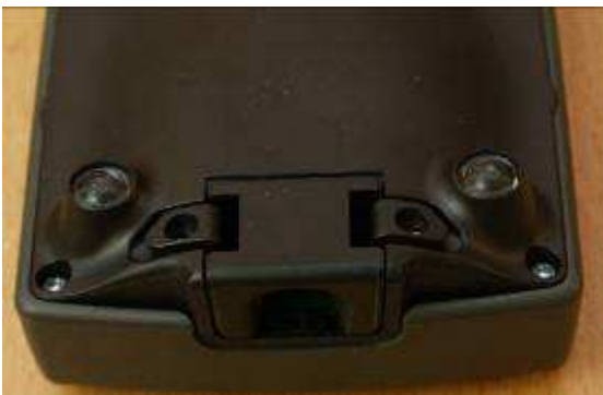
RJ45 Connector with plastic cover
