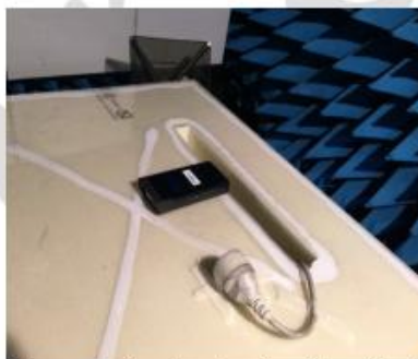
Test setup in anechoic chamber (configuration 2, axis XY)
