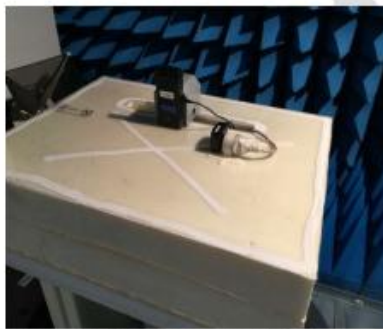
Test setup in anechoic chamber (configuration 1, axis Z)
