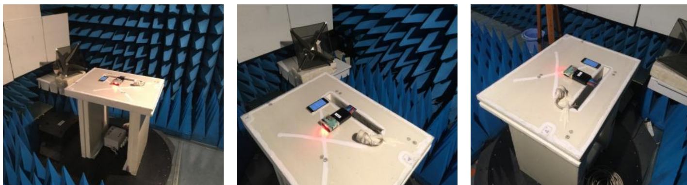
Test setup in anechoic chamber (configuration 2 and axis Z):
