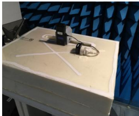
Test setup in anechoic chamber (configuration 1, axis Z)
