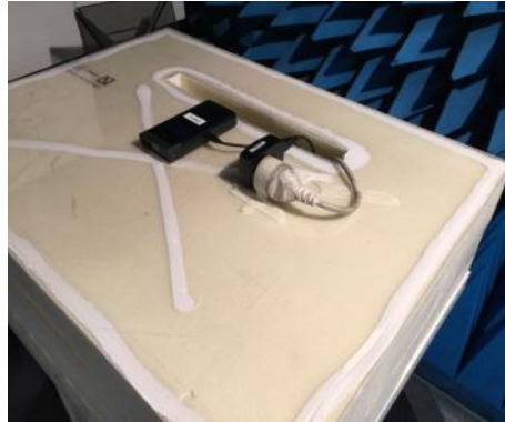
Test setup in anechoic chamber (configuration 1, axis XY)
