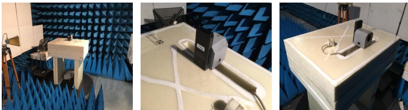
Test setup in anechoic chamber (configuration 2, axis Z)
